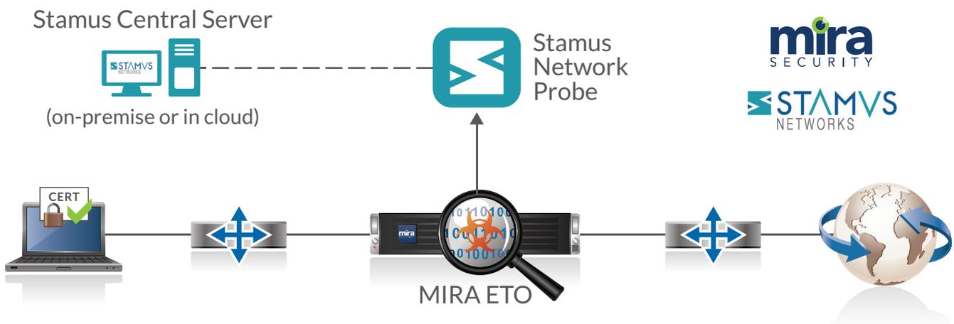
In a "network inline - appliance passive" configuration, the ETO sits in the middle of the traffic flow between the client and the server. When the SSL/TLS handshake occurs, the ETO actively participates in the handshake to insert itself in the TLS flow, it then decrypts the flow and passes the plaintext data over to the Stamus Network Probe for analysis. Then it reencrypts the data and sends it on to the destination, maintaining the end-to-end connection in an encrypted form.
