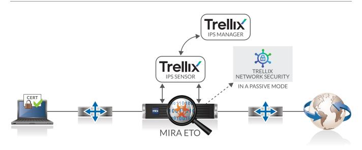
Another Inline-Inline Option: A Defense-in-depth Deployment to Reach Optimal Security Levels As an important feature, Mira's ETO can maintain the previous deployment and add an extra layer of defense by activating the mirroring mode which will be sending decrypted traffic simultaneously to both Trellix's IPS sensor and Trellix's NX running in a passive mode.
